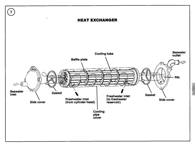
coolant travels to the heat exchanger, where the heat absorbed from engine operation passes through the parallel copper tubes to the water in the seawater system.
