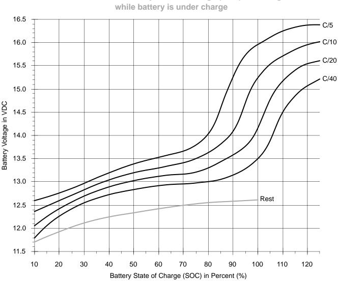
12 Volt Lead Acid Battery State of Charge (SOC) vs. Voltage
