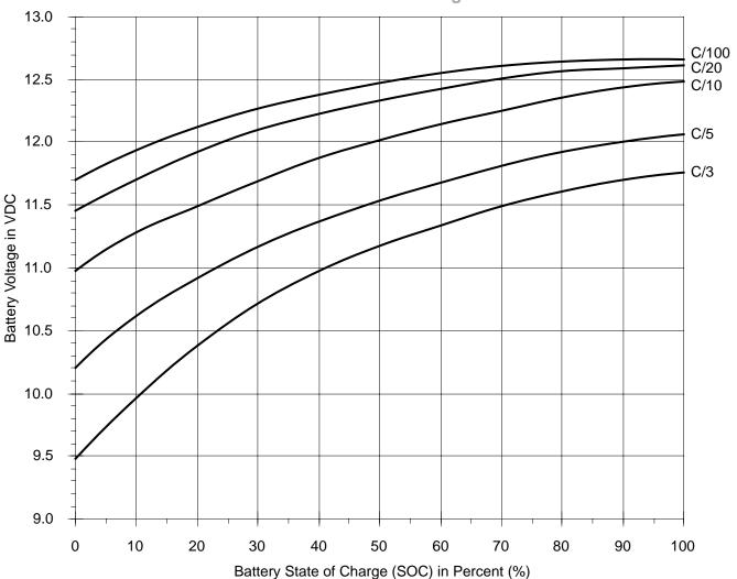
12 Volt Lead Acid Battery State of Charge (SOC) vs. Voltage while under discharge
