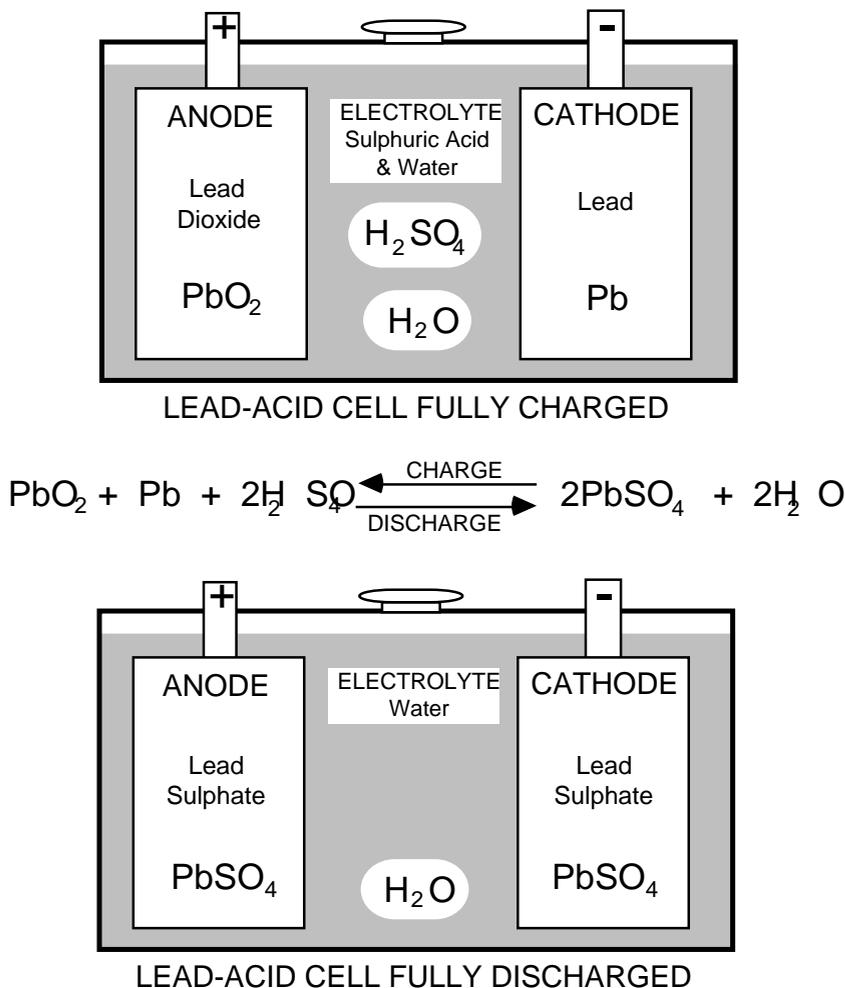
Figure 1- An electrochemical schematic of the lead-acid cell.
