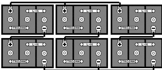
Lead-Acid Battery-- 12 VDC at 1,050 Ampere-hours.
